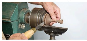
**9.** Using a parting tool, separate the base from the block. Make the cut slightly concave, using a sharp parting tool and remove stock until only 1/2" or so remains. At this point, stop the lathe and saw the rest of the way, or continue grasping the stem and part the rest of the way off.
