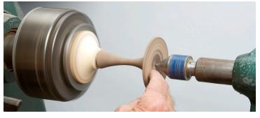
**11.** Turn the bottom of the stem until it's clean and smooth. Sand the base.
