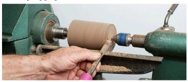
**2.** Square both ends of the blank using the long point of skew chisel flat on its side.
