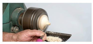
**10.** Use a piece of scrap wood, turn it round and mount it in a chuck. Turn a tenon about 3/4" long and approximately 7/16" in diameter on the blank. Turn or sand the tenon so that it fits snug inside the opening at the top of the stem.
