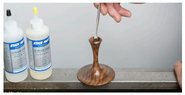
**14.** Apply epoxy to the hole and tapered opening of the wood base, spread evenly.
