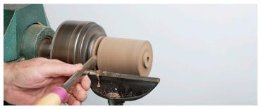
**5.** Cut a 3/4" diameter by 1/4" long shoulder around the drilled opening. Make a 3/4" deep part on the base of the piece approximately 3 3/8" from the drilled end. This indicates the overall length of the stem.
