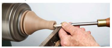
**6.** Rough out the basic shape of the stem, then use a 3/8" spindle gouge to flare the top of the stem to accept the glass. Make light cuts and check the fit frequently, as a good fit is critical for alignment and appearance. The wood should fit tight against the glass.
