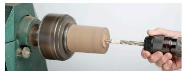
**4.** Using a drill chuck mounted in the tailstock, drill a 7/16" diameter hole, 3/4" deep in the blank. The hole may need to be slightly larger or deeper, as the glass is hand blown and each stem may be slightly different in size.
