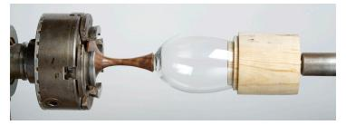
**15.** Mount the goblet base in the chuck and tighten the jaws until they lightly contact the rim. Do Not Over Tighten- as the jaws may mark the wood.
