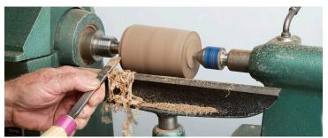
**3.** Cut a 1 3/4" diameter tenon 1/4" to 3/8" long on the end of the blank. The tenon should be slightly tapered so it will fit securely in the chuck jaws. Mount the blank in a chuck.
