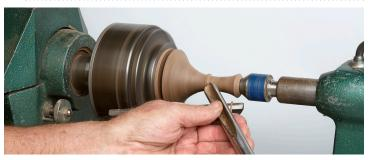
**7.** Using a spindle gouge, shape the stem making light cuts. The stem should not be smaller than 3/8" diameter at the narrowest point. Reduce the base of the stem to 2 3/4" diameter.
