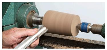
**1.** Select a block 3" x 3" x 4" long. A close-grained wood with straight grain through the stem is recommended. Mount the blank between centers on the lathe and turn it until round using a roughing gouge.
