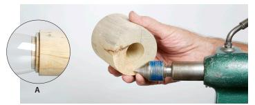
**13.** With the stem set aside to dry, turn a jig that will align and hold the glass in place while the adhesive cures. To do this, turn a cylinder 3 1/2" diameter by 4" long between centers. Drill a hole in one end of the cylinder to fit over the revolving center. Turn a tenon on the opposite end of the cylinder to fit snug inside the goblet opening (see figure A).
