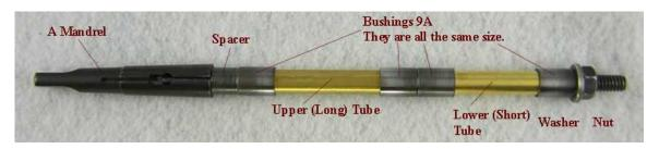
1. Assemble the blanks on the mandrel using the 9A bushings. Selection of the bushings is easy since they are all the same size. Put any bushing in any position.
