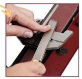
When the first side has been sharpened turn the skew over and place it against the other side of the jig and continue as before, until the tool is razor sharp.
