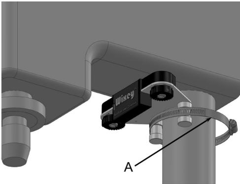
3. Adjust the X-Y position of the lines using Knobs (B) and the Z position using screws (C)
