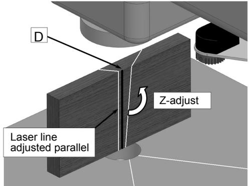
6. Lay the block of wood face down and hold it in position so it doesn't move.
