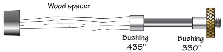
2. Advance a 60° revolving cone center into the dimpled end of the mandrel and tighten using light pressure. **Do Not** over tighten the tailstock or mandrel nut as this may cause the mandrel to flex resulting in off-center barrels.
