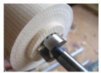
Pedestal to receive the base plate, 25 mm (1") bore for the nutmed
