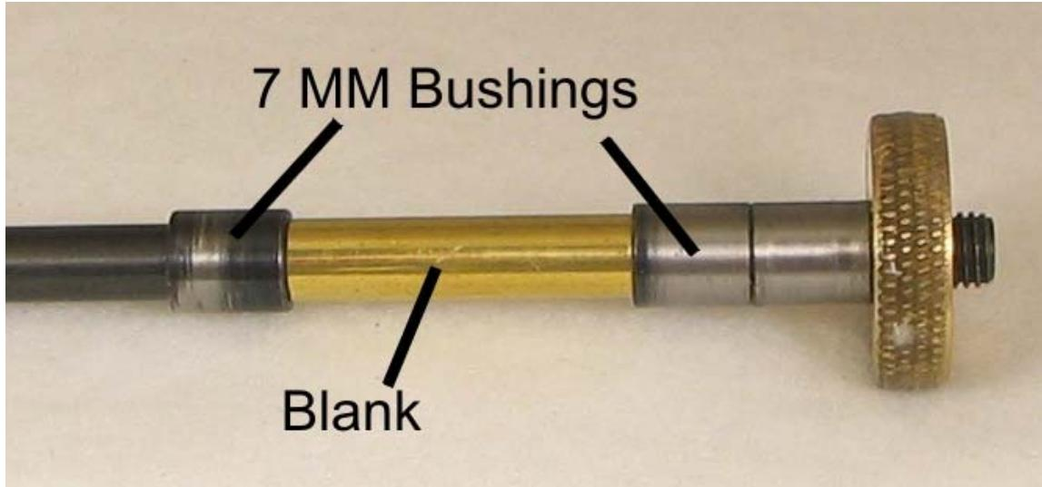
1. Assemble the blank on the mandrel using 7 MM bushings. With these bushings it is not necessary to be particular with the order they go on the mandrel. They are all identical. It will take a large spacer to take up the space on the mandrel. You can use an old blank or extra 7 MM bushings or a combination of the two.
