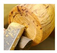
the insert. Scribe the end of the stopper using the sharp points of the caliper to indicate the diameter of the recess required for fitting the insert. *Hint: When scribing the stopper, do so with the lathe turning at a slow speed to prevent a catch.*
