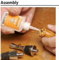
**3.** Using a flexible instant glue or RTV silicone adhesive, place a small amount of adhesive in the recess and press the insert firmly into place.
