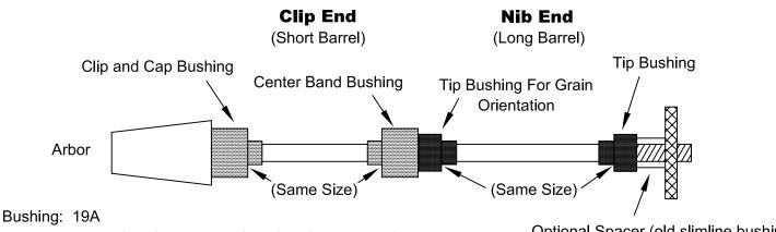
Drills needed: 15/32" (upper barrel), 25/64" (lower barrel) Blank size: 3/4" x 3/4" x 5" long
