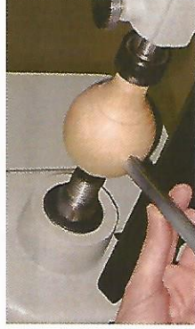
Pin to hold the mill body
